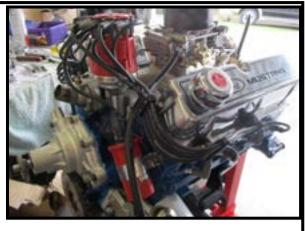
The original MSD distributor was used, with the addition of heatproof socks, to prevent burning of the leads on the headers.
